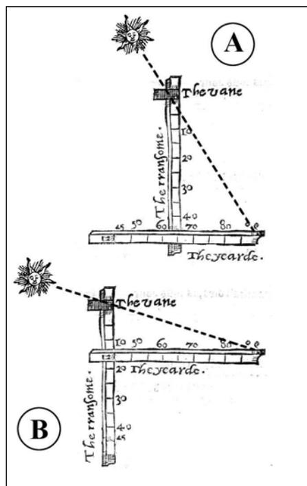
Fig. 9 Using Hood's staff according to Hood and Blundeville.<sup>70</sup>
