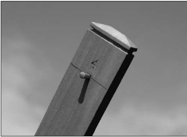
Fig. 10 The upper end of the cross of the reconstruction showing one of the pins and the corresponding scale number.
