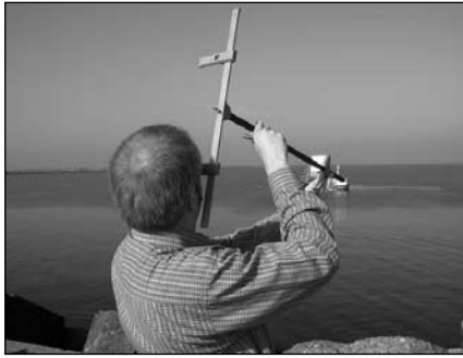
Fig. 4 The author with the spiegelboog re-construction set up for bright sun observations.
