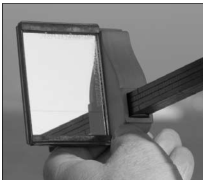
Fig. 11 The mirror-vane of the reconstruction with the mirror attached.
