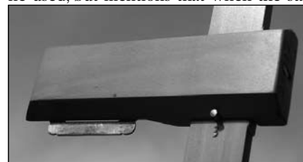
Fig. 17 The sight-vane of the reconstruction with the aperture at pin number 3.
