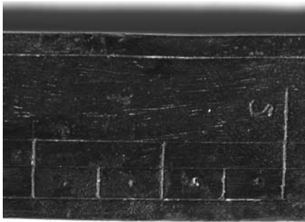
Fig. 15 Detail of the Kennemerland hoek-boog scale showing the divisions from 3 degrees (left) to 5 degrees (right) and their subdivisions.
