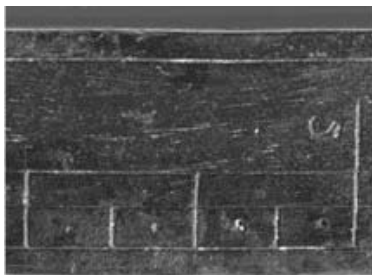
Fig. 24 Detail of the Kennemerland hoekboog scale showing the divisions from 3 degrees (left) to 5 degrees (right) and their subdivisions.
